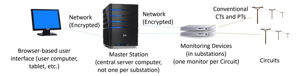
This monitoring system provides high resolution, sensitive triggering, and long records. It is installed on more than 600 circuits and detected the field case discussed in this presentation.
