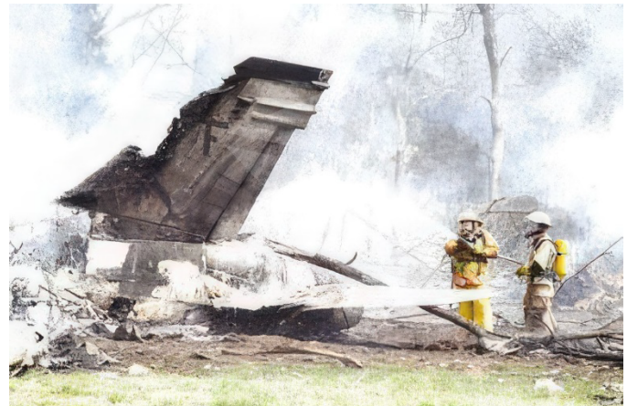
Fig. 12. Vertical stabilizer showing damaged areas where the stabilizer contacted the power conductors [6] (image used by permission).
