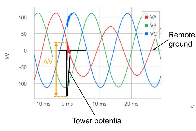
Current TW is significantly higher than the point-onwave voltage would allow
