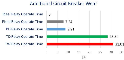
Fig.12 Additional circuit breaker wear comparison [7]
