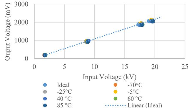
Fig. 13. Temperature Impact Test Results for Voltage Sensor B
