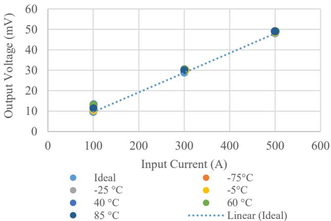
Fig. 11. Temperature Impact Test Results for Current Sensor B
