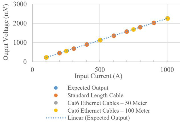
Fig. 6. Linearity and Accuracy Test Results for Current Sensor A
