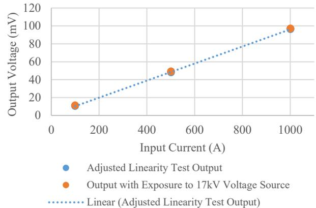
Fig. 17. EMI Impact Test Results for Current Sensor B
