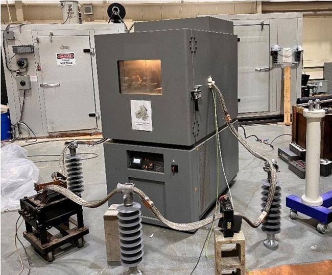
Fig. 4. Setup for Testing Temperature Impact Using the Temperature Chamber
