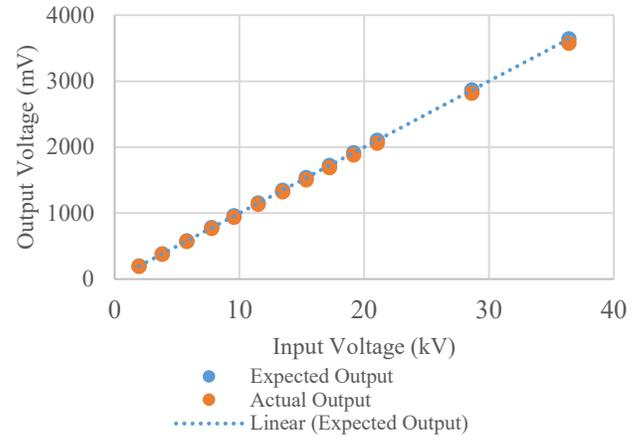
Fig. 8. Linearity, Accuracy, and Withstand Capability Test Results For Voltage Sensor A
