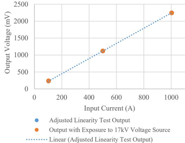
Fig. 16. EMI Impact Test Results for Current Sensor A
