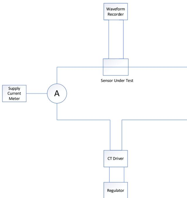
Fig. 1. High-Level Layout of Test Setup for Testing the LPIT Current Sensors
