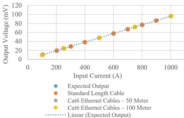
Fig. 7. Linearity and Accuracy Test Results for Current Sensor B
