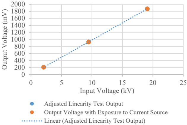
Fig. 19. EMI Impact Test Results for Voltage Sensor B
