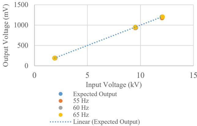
Fig. 14. Frequency Impact Test Results for Voltage Sensor A
