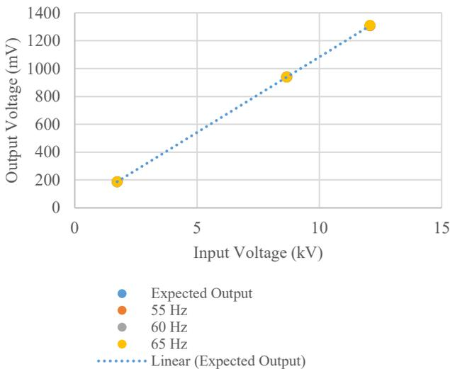
Fig. 15. Frequency Impact Test Results for Voltage Sensor B
