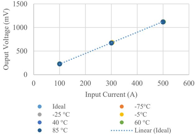
Fig. 10. Temperature Impact Test Results for Current Sensor A
