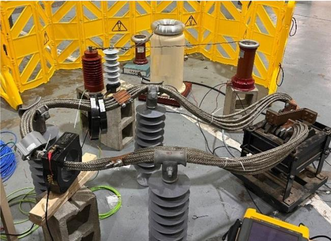
Fig. 5. Setup for Impact of Electromagnetic Interference Testing
