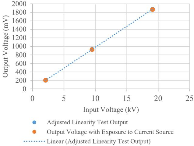
Fig. 18. EMI Impact Test Results for Voltage Sensor A
