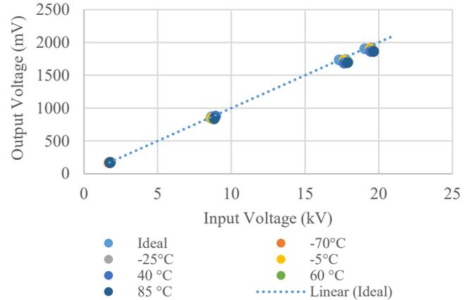
Fig. 12. Temperature Impact Test Results for Voltage Sensor A
