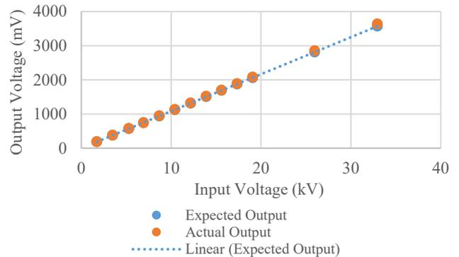
Fig. 9. Linearity, Accuracy, and Withstand Capability Test Results for Voltage Sensor B
