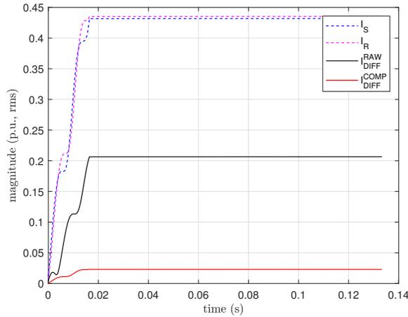
Fig. 7. Voltage-based charging current compensation in two-terminal fully untransposed transmission line.
