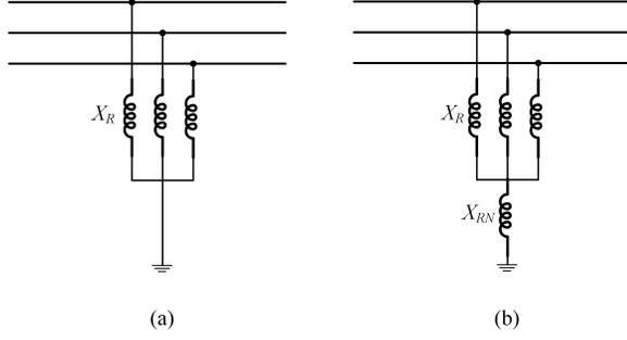
Fig. 10. (a) Three-reactor arrangement (b) Four-reactor arrangement.
