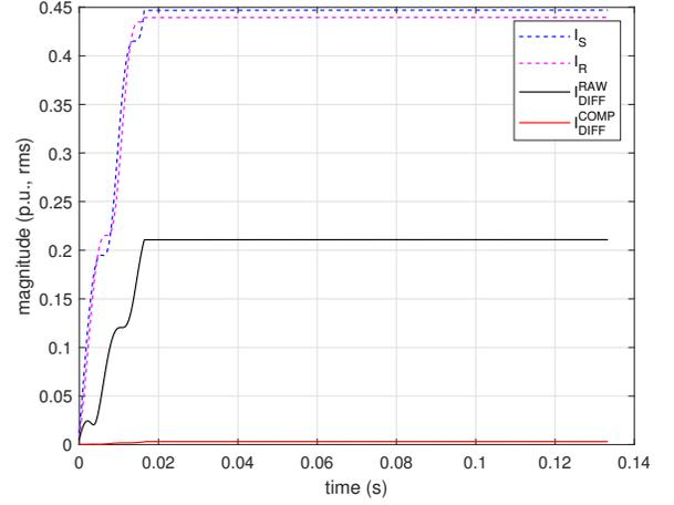
Fig. 6. Voltage-based charging current compensation in two-terminal fully transposed transmission line.
