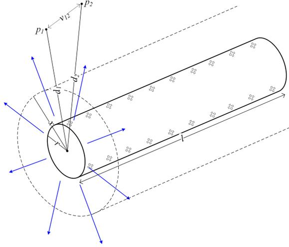
Fig. 1. Electric field due to a cylindrical charged conductor.
