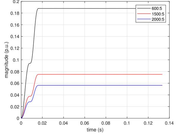
Fig. 11. Charging current of an 80km, 500kV transmission line measured through different CT ratios.
