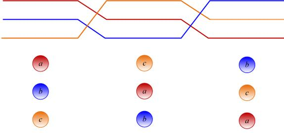
Fig. 4. Transposition of the transmission line.
