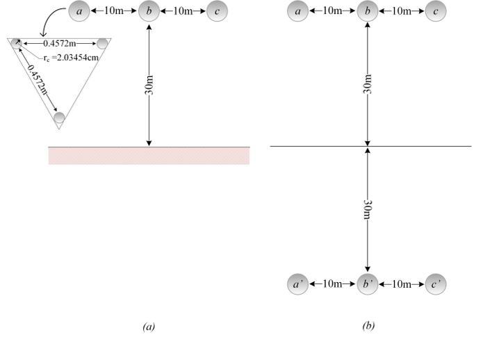
Fig. 3. A three phase conductor arrangement on a tower: (a) over the earth surface plane, (b) earth replaced by a perfect conducting surface plane showing mirrored conductors.
