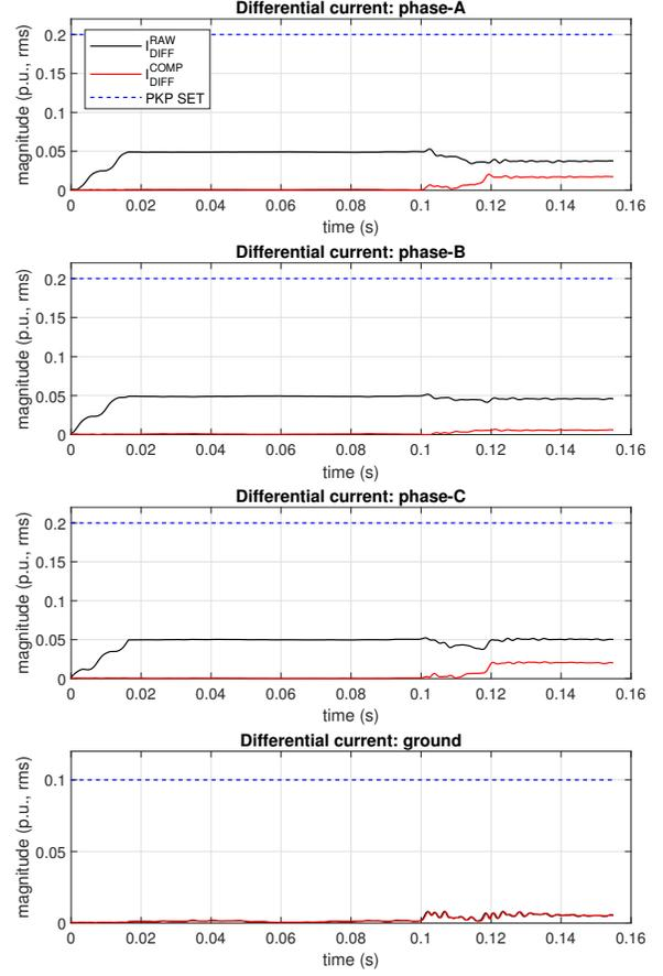
Fig. 13. Field Case of an external ACG fault: Raw and compensated differential current in phases-A, B, C and ground channel.
