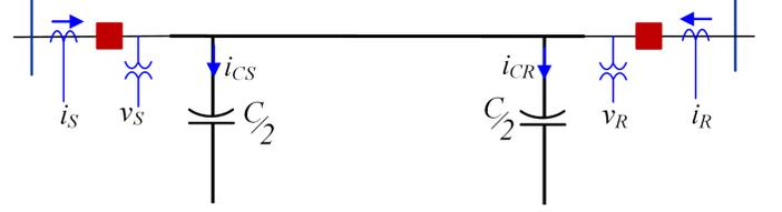
Fig. 5. Voltage-based charging current compensation in two-terminal transmission line.
