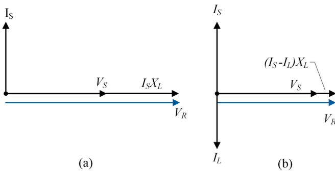
Fig. 8. Phasor diagram depicting: (a) Ferranti effect, (b) remediation through shunt reactors.
