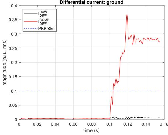
Fig. 12. Field Case of an external ACG fault: Raw and compensated ground differential current.
