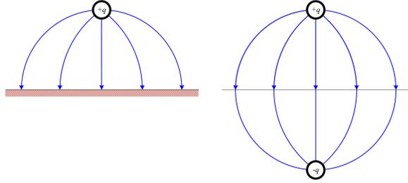
Fig. 2. Effect of earth on the electric field due to a cylindrical charged conductor.
