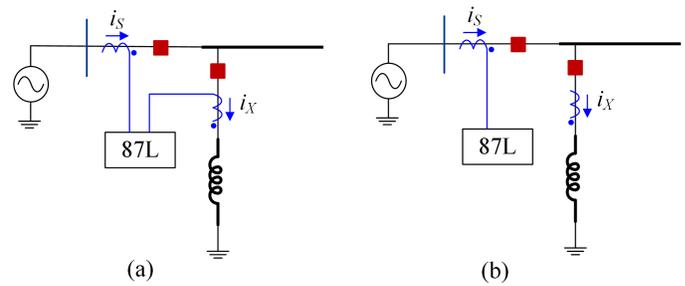
Fig. 9. Reactors connected to transmission line: (a) excluded from the protection (b) included in the protection Zone.
