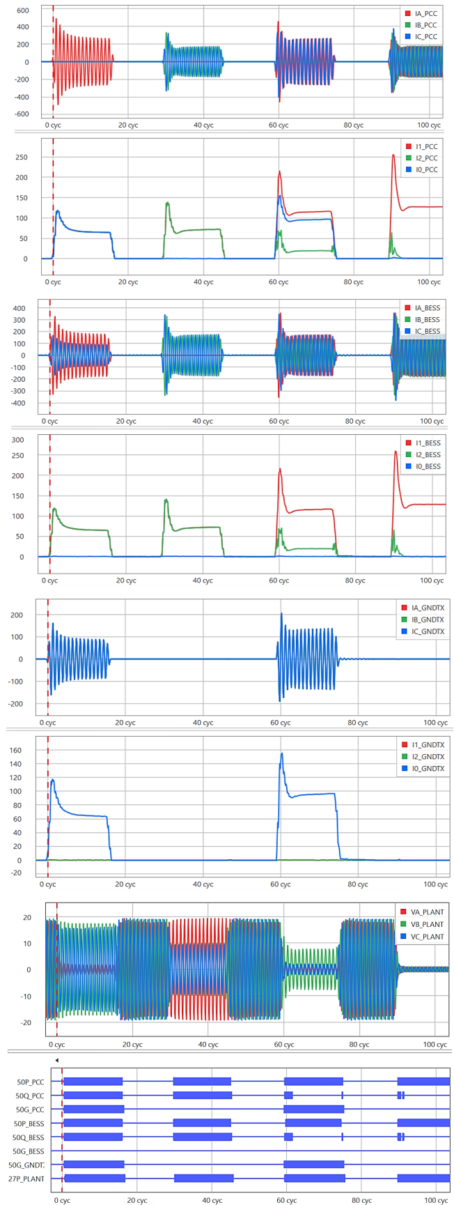
Fig. 8 Phase and Sequence Fault Currents at the PCC, BESS, and Grounding Transformer Breakers, Plant Bus Voltages, and Digitals
