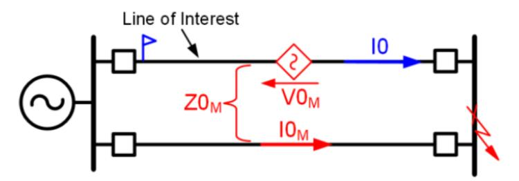
SOURCE IMPEDANCE RATIOS FOR GROUND FAULTS: OUTAGE Vdrop (V) Irelay (A) Vdrop/Irelay (ohm) SIR None 61861.9 1290.41 47.9397 5.054
