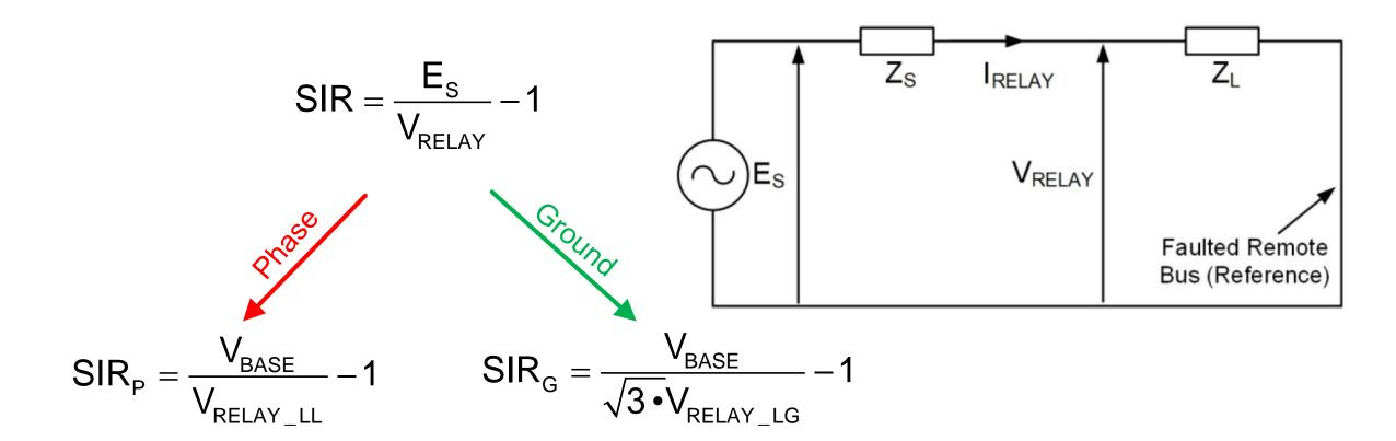
Uses loop voltage directly as used by the 21P element ( $V_{LL}$ ) and 21G element ( $V_{LG}$ )!
