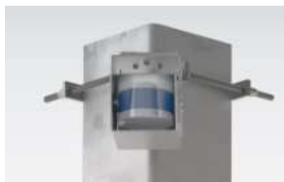
Fig. 8. LiDAR sensor mounted on transmission-tower strut
