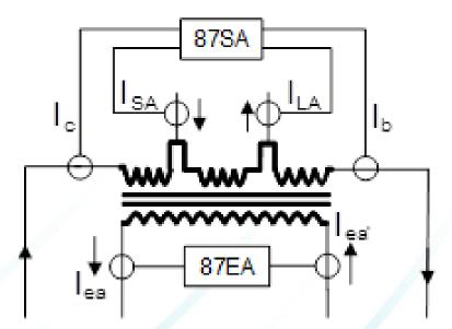
Method 2 – Two ends currents-based method that can be applied to Any PST Type
