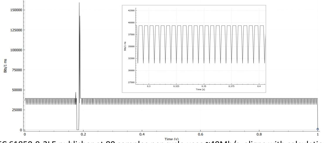
8 IEC 61850-9-2LE publisher at 80 samples per cycle uses ~40Mb/s, aligns with calculations
