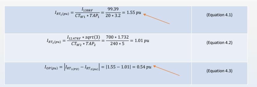
Note: Primary side contribution is 1,100 A on the 12.47 kV side (400 A + 700 A) reflected to 138 kV.
