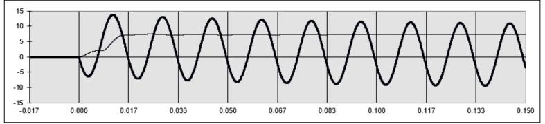
Used PSRC CT Saturation Calculator to model the Breaker 8 (I<sub>2</sub> current) CT that sees almost all the fault current
