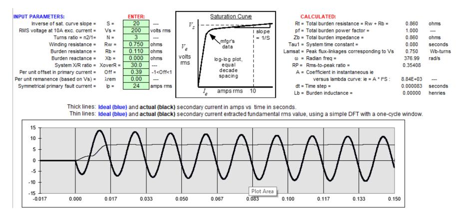
No saturation for this fault event – will faithfully reproduce the output of the bushing CT.
