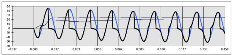
C200 tapped down to 50% winding (effectively a C100), high connected burden
