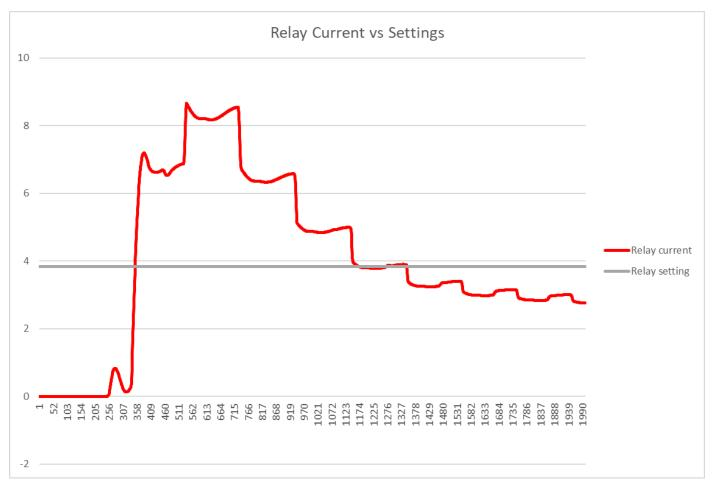
Used a 1-cycle DFT to calculate a phasor quantity for the CT error current
