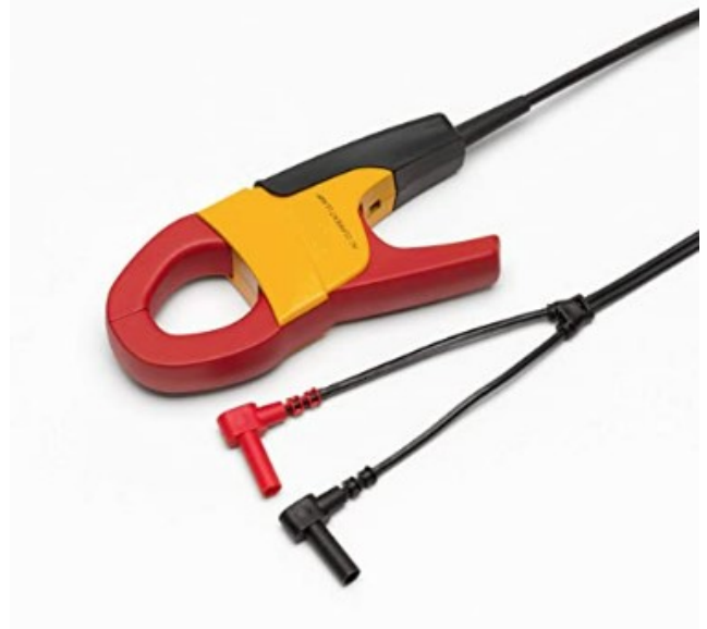
Fig. 10. Amp clamp meter to verify de-energization of a CT circuit
