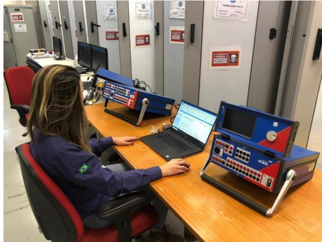
Figure 8. Picture during SE Lorena's 87B SAT (no analog connections)
