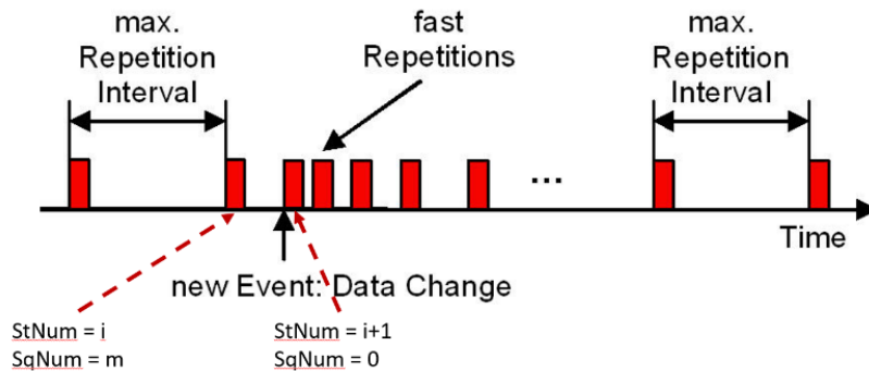
Fig. 2 GOOSE repetition mechanism
