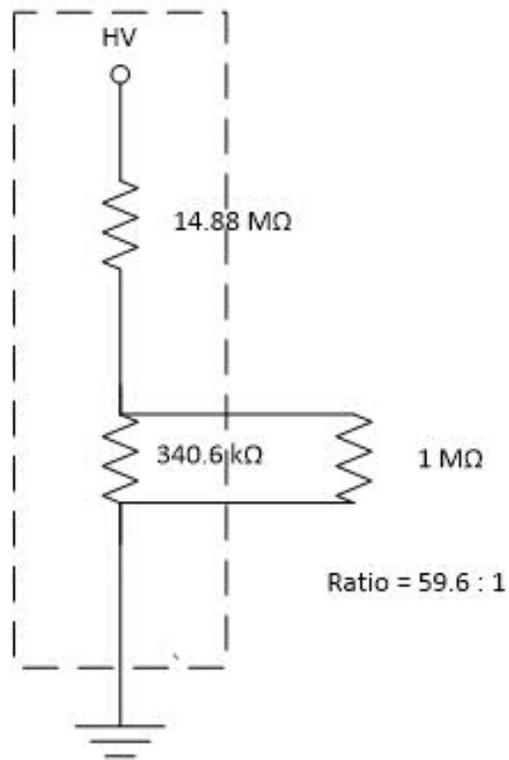
Tuned to a ratio of 60:1 when the device connected to the voltage divider output has an input resistance of  $1 \text{ M}\Omega$
