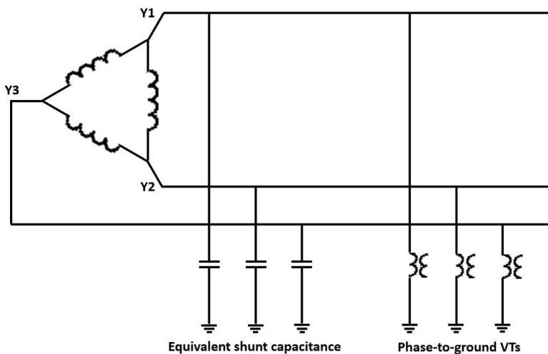
Ferroresonance oscillations → may lead to higher phase-to-ground voltages → repetitive saturation → high currents → heating → eventual failure of the VT
