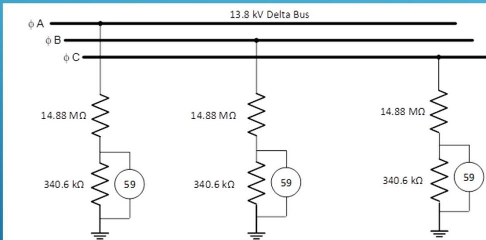
Uses resistive voltage divider, per phase
