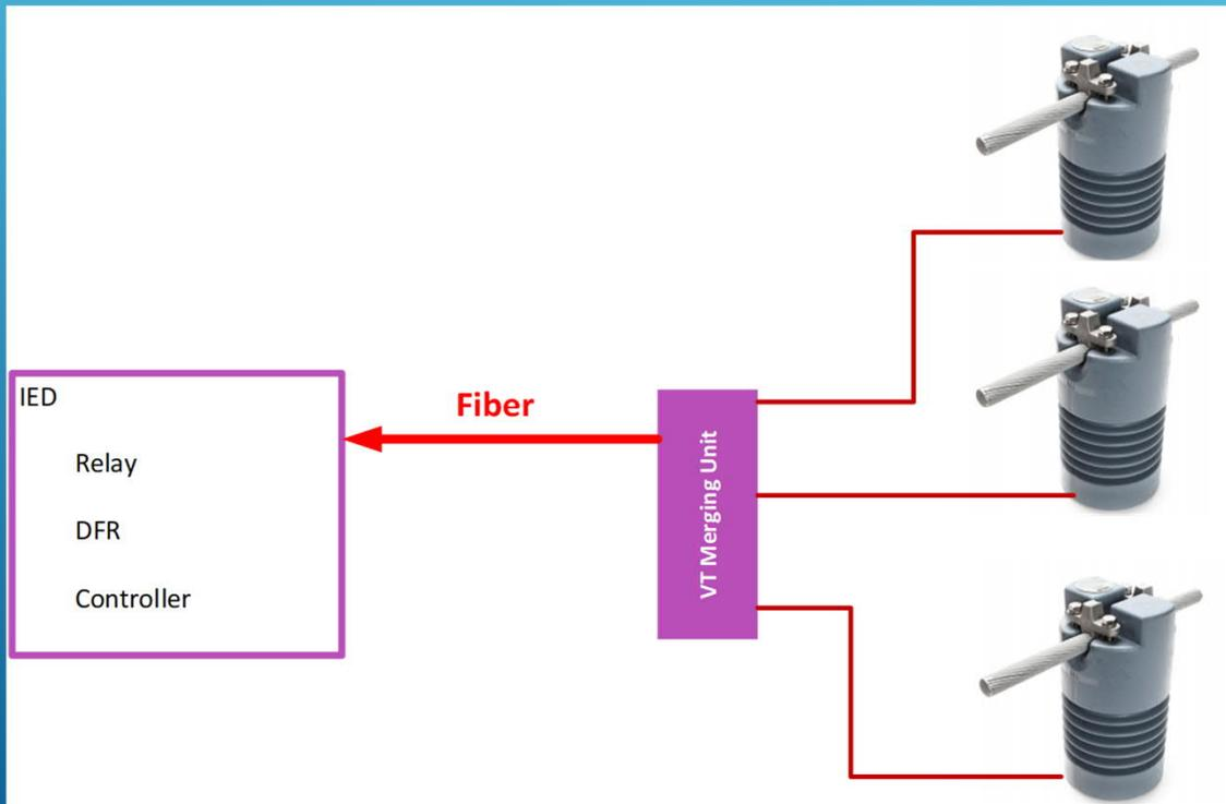
VT-MU located close to the voltage divider
