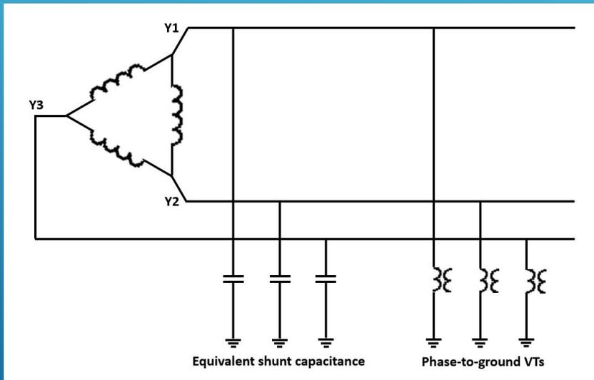
A ground fault on an ungrounded network will produce very little ground fault current
