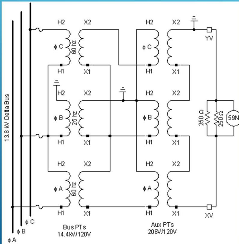
BPA developed and applied a unique voltage sensing scheme
