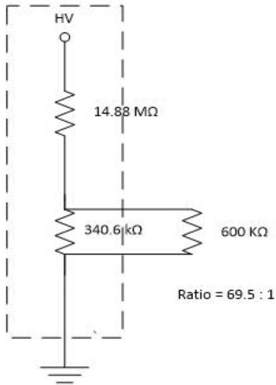
The ratio will change when the device connected to the voltage divider output has an input resistance different from  $1 \text{ M}\Omega$
