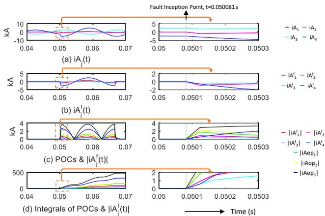
Fig. 3. A-G internal fault event
