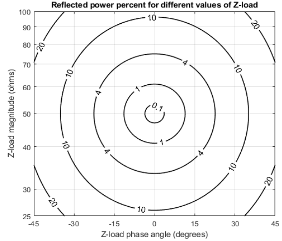
Fig. 8. Contour map of complex impedance Z_{LOAD} versus reflected power for Z_{SOURCE} = 50 ohms, 0 degrees
