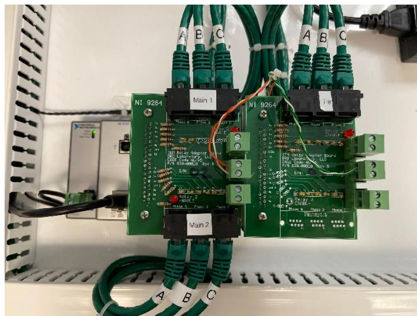
Simulated aCT and VD signals coming from the custom relay adaptor board
