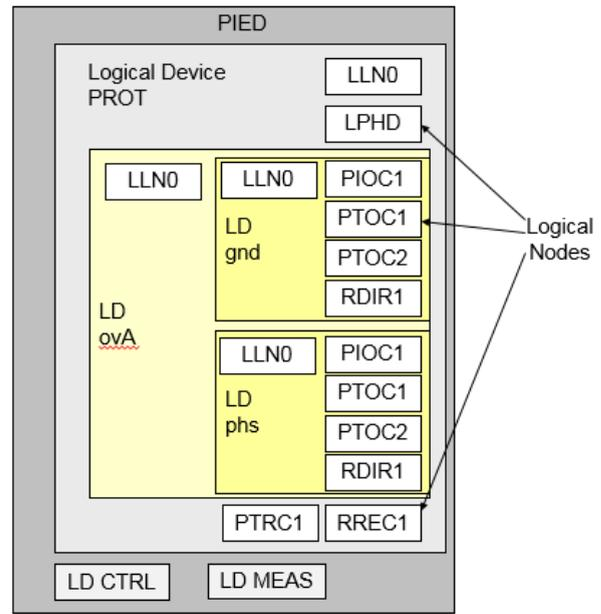
Fig. 5 Logical device hierarchy – simplified object model
