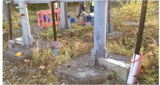
Fig. 12. Primary measurement of I_p with 4 Rogowski coils
