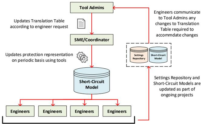
Fig. 8. Update process for protection representation and Translation Table
