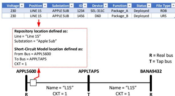
Fig. 3. Different naming conventions for the same location
