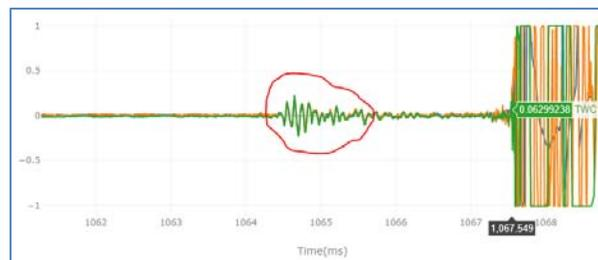
Figure 4, Real measured traveling waves at both terminal
