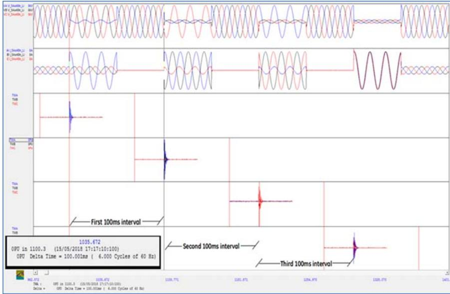
Figure 7, Hardware in the Loop simulated signals showing TWFL solution for consecutive faults
