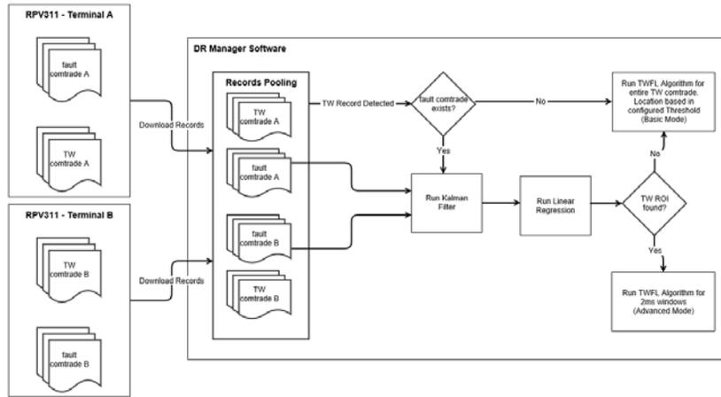
Figure 5, Concentrator Software flowchart for TW-based fault location
