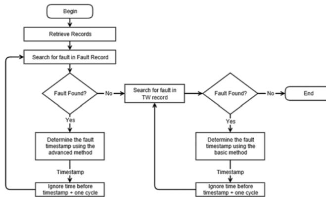
Figure 8, Flowchart for evolving faults location
