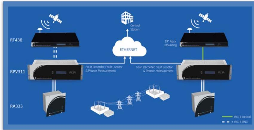
Figure 2, Architecture for traveling-wave-based fault location solution
