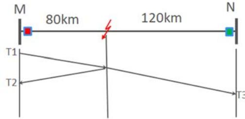
Figure 9, The traveling wave propagation
