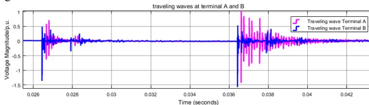
Figure 6, the signature of traveling wave for external phase A to ground fault evolving to internal phase AC to ground fault
