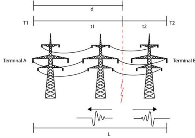
Figure 1, Traveling Waves propagation in a line.
