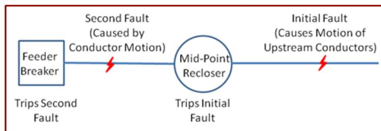
In summary, what begins as a routine fault that should trip only a mid-point protection device instead escalates into a fault of higher amplitude, closer to the substation, and often necessitates circuit-wide interruption.
