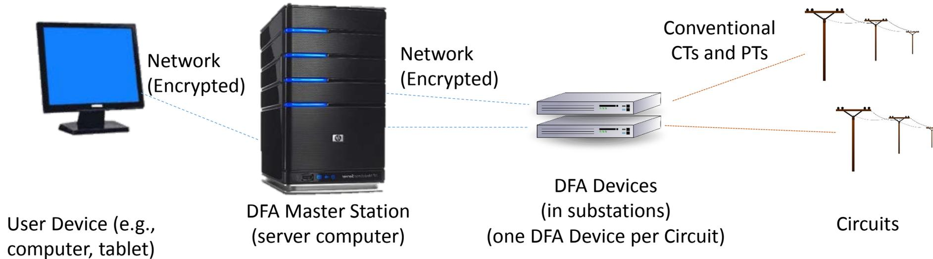
Each substation-installed DFA Device runs waveform analysis and classification software and then sends results to a central DFA Master Station. Personnel access DFA results via browser connection to the DFA Master Station.
