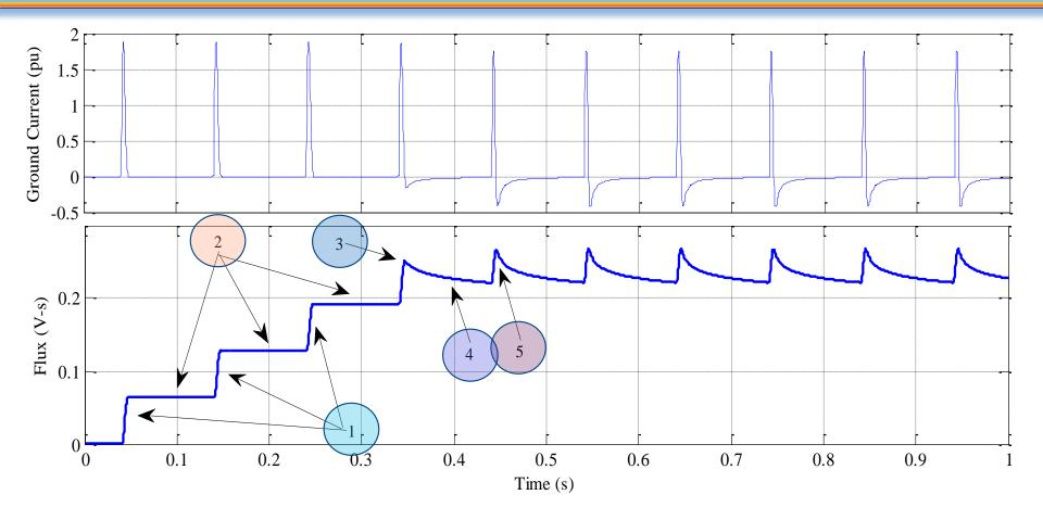
• Stage 5: For the fifth spike and above, the stages 3 and 4 above repeat. The saturation degree becomes stable.
