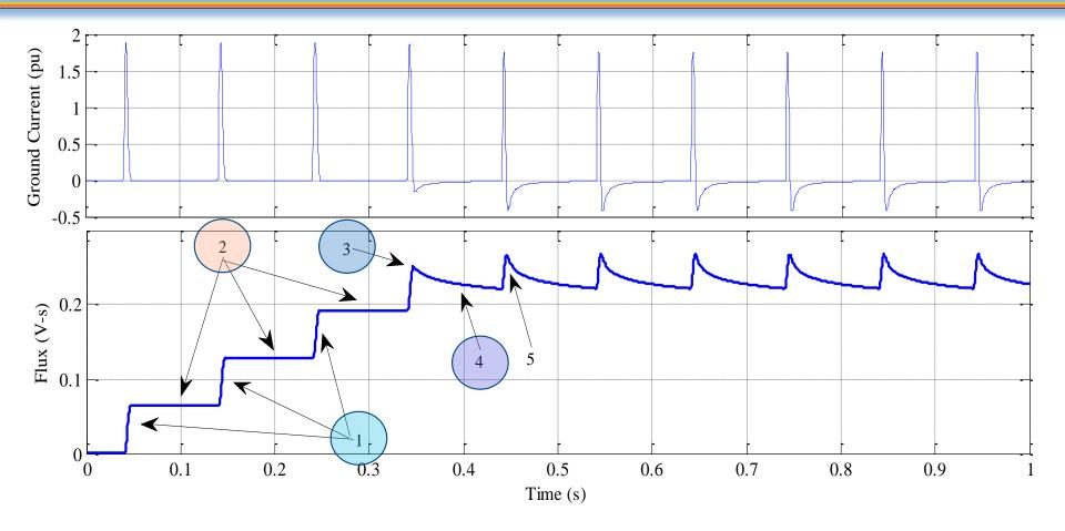
Stage 4: Once entering the saturation zone, the magnetic flux starts decaying to the residual flux level following primary current interruption.
