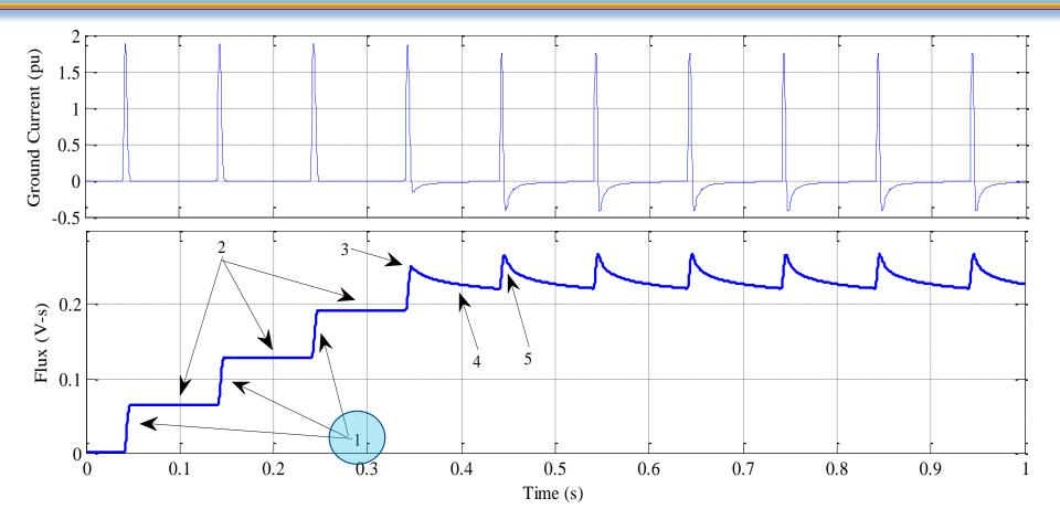
Stage 1: Flux linkage increases when a positive pulse is injected. Each pulse would boost the flux level by 0.0645 V-s.
