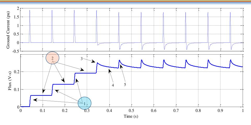
Stage 2: when the injection disappears, the flux linkage would not decay because flux does not exceed the residual flux (around 0.156 V-s).
