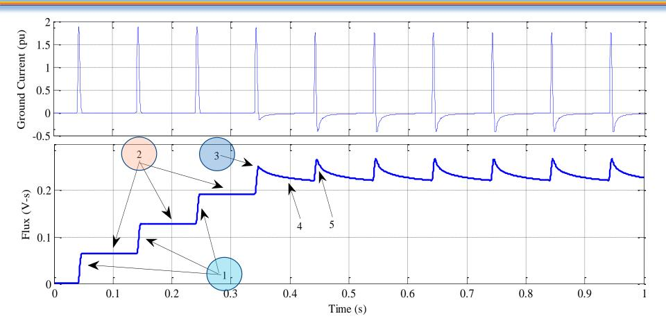
Stage 3: Ground CT enters the saturation because the accumulated flux linkage (0.2512 V-s) exceeds the saturation flux (0.24 V-s).
