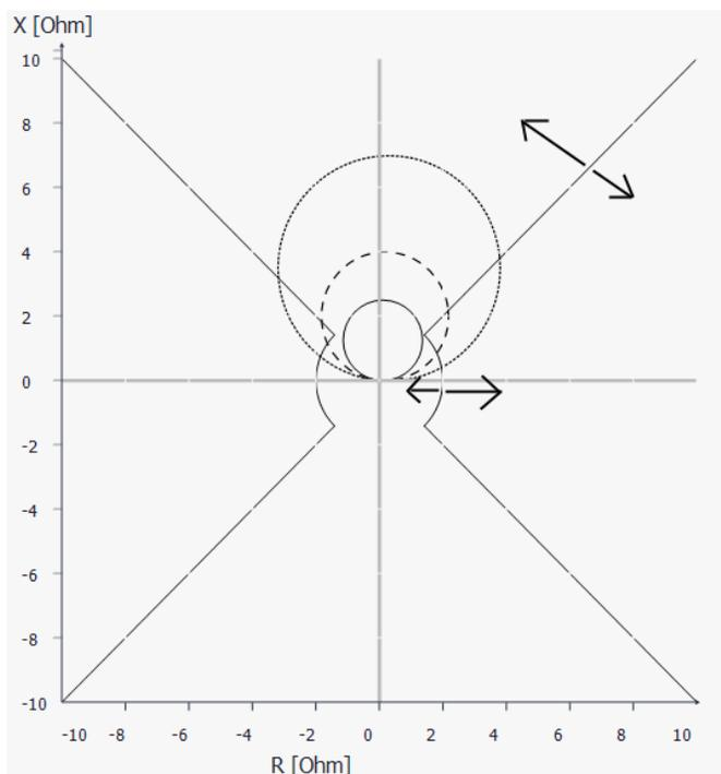
Fig. 3 mho characteristic with load encroachment
