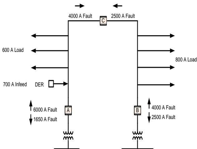
Fig. 1. Distribution system with fault and load currents
